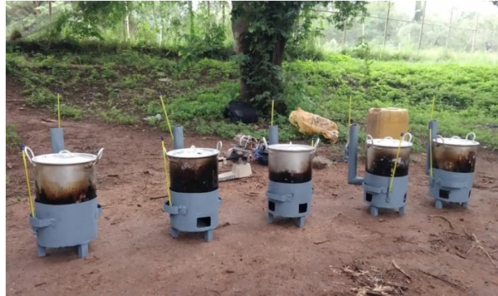
Figure 2.2: View of the five stoves with pots during data collection
