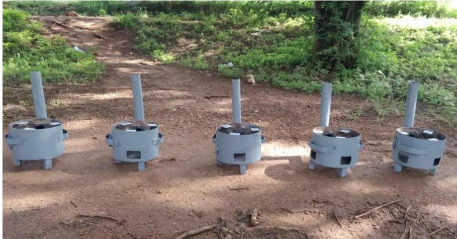
Figure 2.1: View of the five stoves constructed stove with different numbers of air inlets
